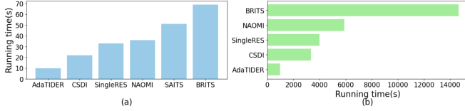
Fig. 4: (a) Average running time for 100 epochs on a 100 \times 100 matrix. (b) Total training time on Westminster-Central.
